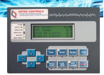
Entek OPI-420 is a combined Operator Interface and Embedded Controller in one complete package. OPI-420 offers a cost effective solution as a versatile display and control device that can be used for a wide range of commercial or industrial applications by Original Equipment Manufacturers. It comes with plug-in input/output module options, and on-board serial ports for auxiliary devices.
